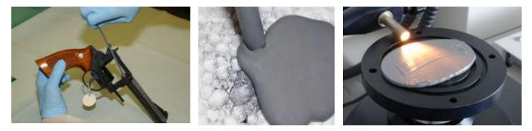
Furthermore, the material is now even more flexible and has a greater tear strength thus reducing the chance of damage when removing imprints from marks.
